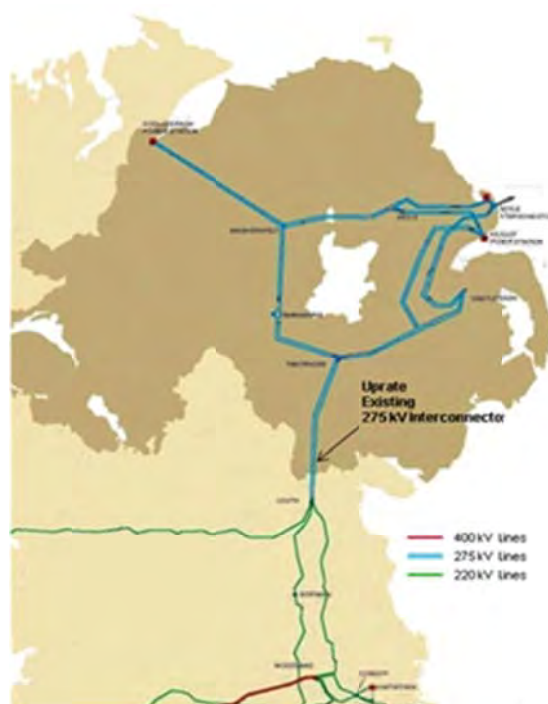
Figure 2.3: Existing High Capacity Transmission Network in the North-East of Ireland
