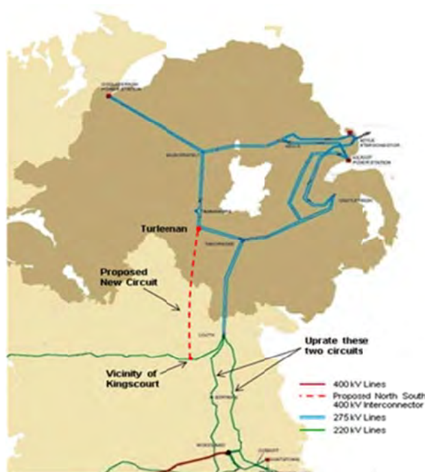
Figure 2.4: Scenario: New Kingscourt-Turleenan Circuit and Up-rating of Existing 220 kV Circuits
